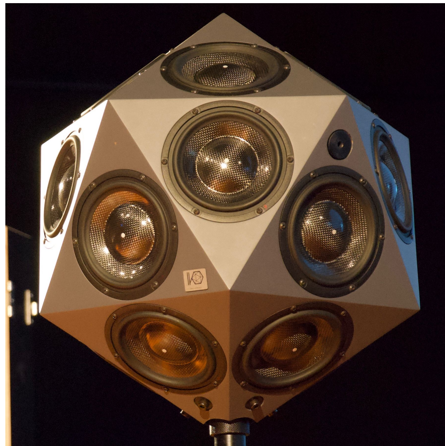
Figure 1: Icosahedral loudspeaker "IKO by IEM and sonible" with about 0.3 m edge length and 20 six-inch drivers, available at iko.sonible.com.
